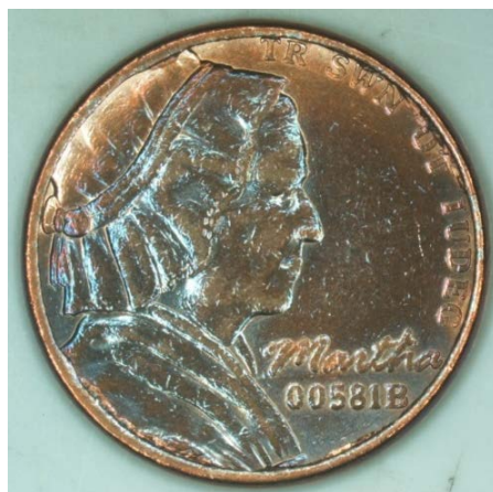
Figure 3-9. CPZ After Wear Test
