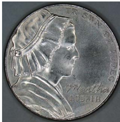
Figure 3-31. 80/20B Test Piece (54T Strike)
