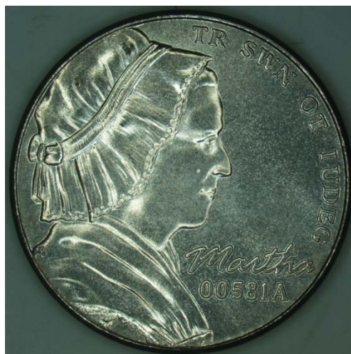
Figure 3-44. 80/20B Test Piece (54T Strike)
