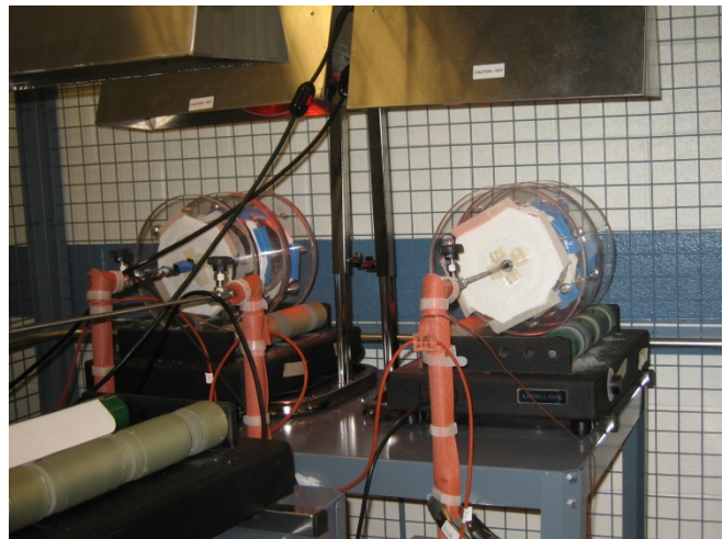
Figure 3-2. Steam Test Tumblers
