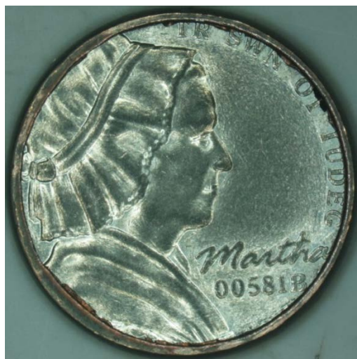
Figure 3-14. TPCPZ After Wear Test
