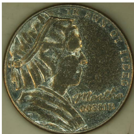
Figure 3-30. 80/20A After Wear Test
