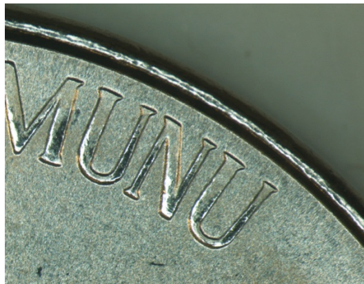
NPS five-cent: edge lettering showing poor letter fill
