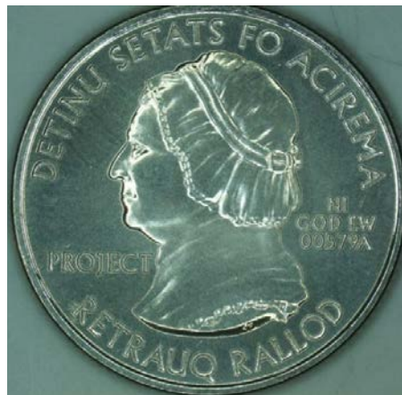
Figure 3-38. NPS Quarter-Dollar Test Piece (66T Strike)
