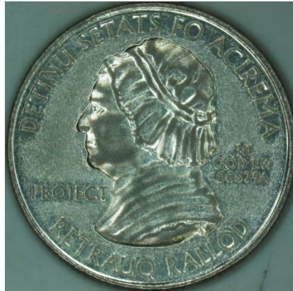
Figure 3-20. MPPS Quarter-Dollar After Wear Test
