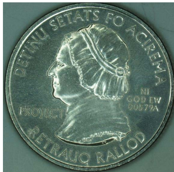
Figure 3-35. MPPS Quarter-Dollar Test Piece (64T Strike)
