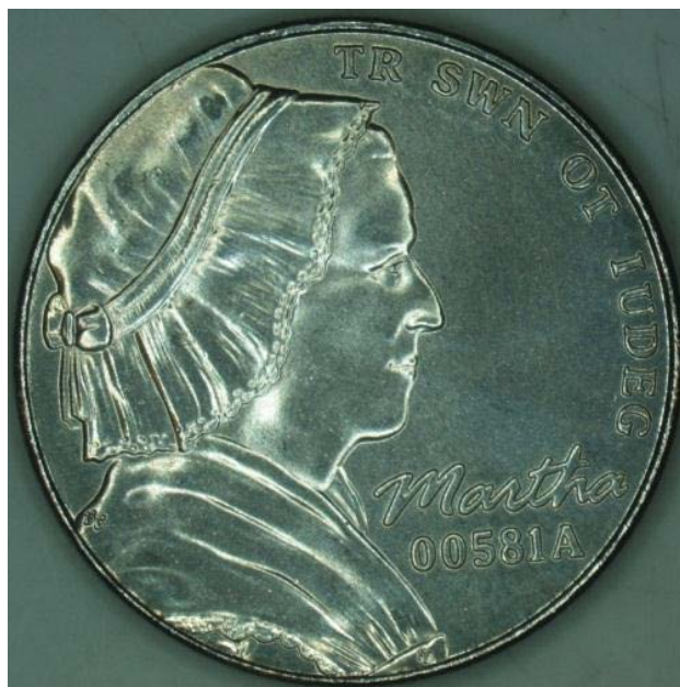
Figure 3-34. MPPS Five-Cent Test Piece (56T Strike)
