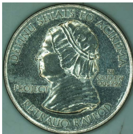
NPS quarter-dollar nonsense piece after wear test
